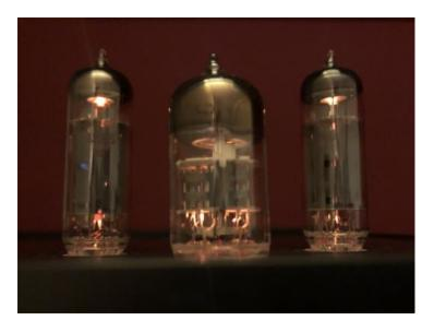
Within about 20-30 seconds from switch on the amplifier will be starting to work (it can take up to 5 minutes to reach full specification).
