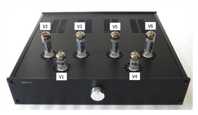
If the valves are correctly installed, the base of the valve will sit flush with the top of its ceramic socket there will be no pins (or virtually no pins) visible and the valve will be vertical – see next picture.
